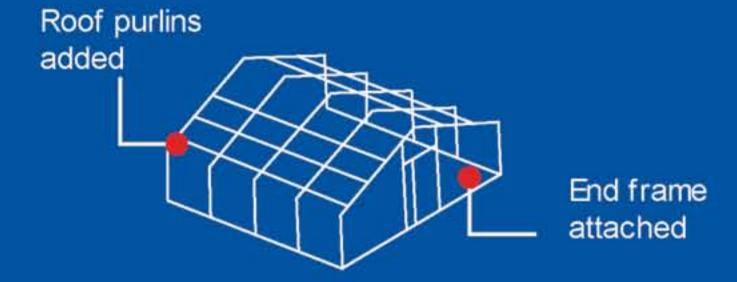
Steel frame members are easily erected in a few hours. Ground anchors are used to secure frame to ground
