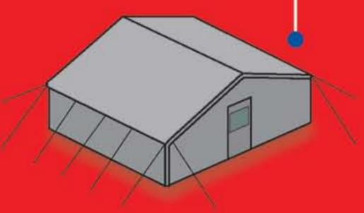
Utilizing a galvanized steel frame, Absolute Steel's Trasitional Relief Housing addresses immediate response needs and then provides the basic frame system for permanent housing as families accumulate the materials - wood, metal sheeting etc. to build onto them.
